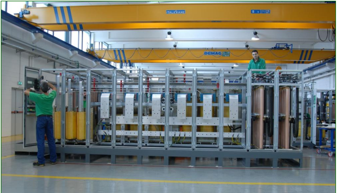
Manufacturing a 500kVA Sirius ...
